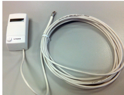
Ambient Sensor version remote sensor with 1 integrated sensor and 1 remote sensor
