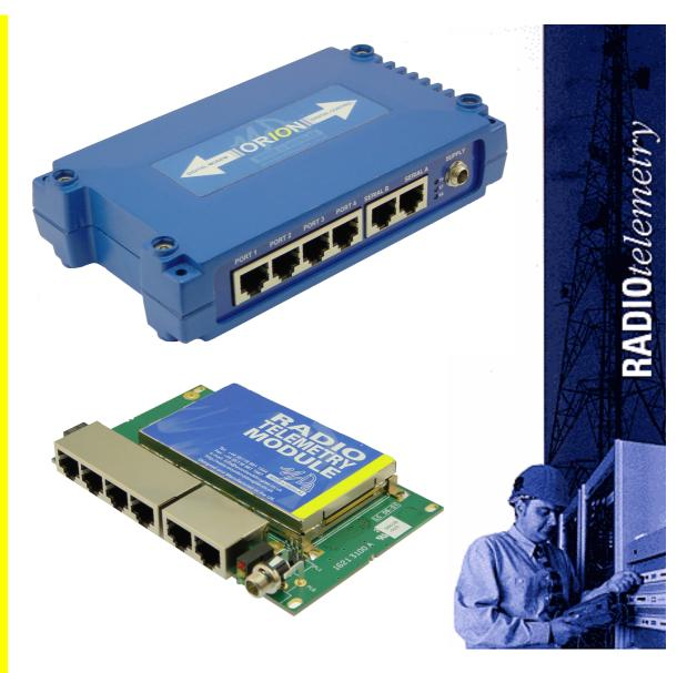
The ORION has a selectable RS232, RS422, RS485 user interface for serial data messaging allowing easy connection to Remote Telemetry Units, Pan Tilt Zoom camera controllers etc. Over-air data rate is 19200bps when a 25kHz bandwidth radio module is fitted (9600bps in a 12.5kHz channel).
